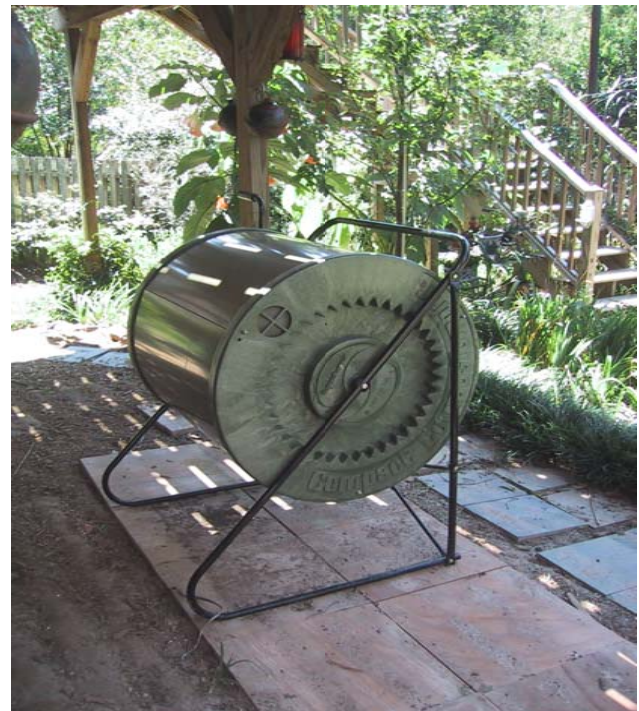
This compost drum must be turned daily with a crank (located on the opposite side of the drum) and can produce humus in as little as three weeks.
